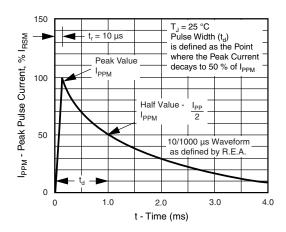
Fig. 3 - Pulse Waveform
