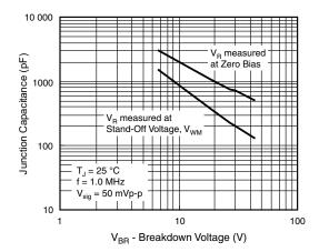
Fig. 4 - Typical Junction Capacitance
