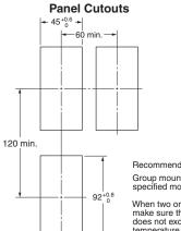
Recommended panel thickness is 1 to 8 mm. Group mounting is not possible. (Maintain the specified mounting space between Controllers.)
