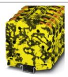
High-current terminal block, Connection method: Push-in connection, Cross section: 25 mm<sup>2</sup> - 95 mm<sup>2</sup>, AWG: 4 - 3/0, Width: 25 mm, Color: black/yellow, Mounting type: NS 35/15
