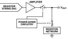
Figure 35. Output Stage During Power-Down
