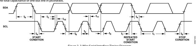
Figure 2. 2-Wire Serial Interface Timing Diagram
