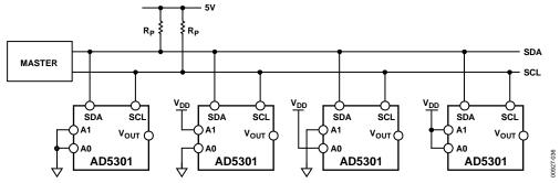
Figure 38. Multiple AD5301 Devices on One Bus
