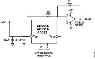
Figure 37. Bipolar Operation with the AD5301/AD5311/AD5321
