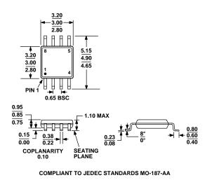
Figure 40. 8-Lead Mini Small Outline Package [MSOP] (RM-8) Dimensions shown in millimeters
