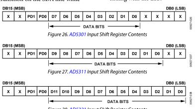
Figure 28. AD5321 Input Shift Register Contents
