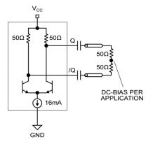
Figure 11. CML AC-Coupled Termination
