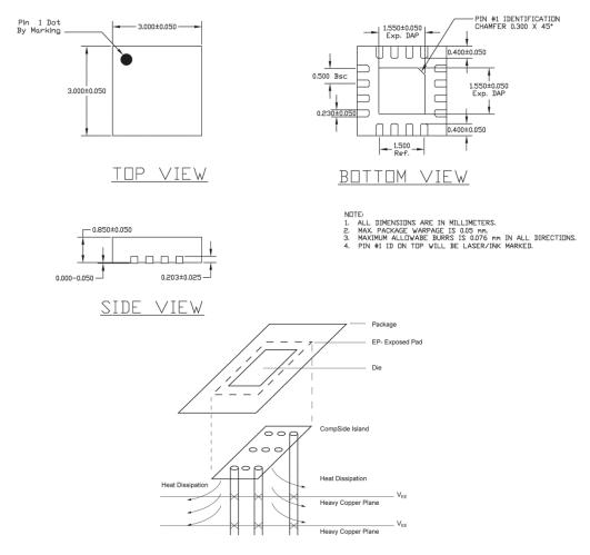
PCB Thermal Consideration for 16-Pin QFN Package (Always solder, or equivalent, the exposed pad to the PCB)
