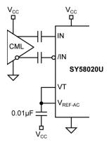
Figure 5. AC-Coupled CML Input Interface
