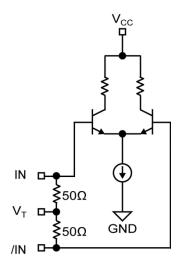
Figure 3. Simplified Differential Input Buffer
