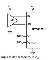
Figure 4. DC-Coupled CML Input Interface
