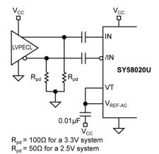
Figure 9. AC-Coupled LVPECL Input Interface
