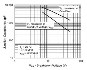
Fig. 4 - Typical Junction Capacitance
