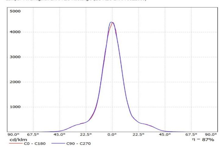
Luminaire: Ledil Oy CN12603\_LENINA-S-DL\_(BXRA\_ES\_Rectangle)\_SIMULATED Lamps: 1 x Bridgelux BXRA ES Rectangle (ES-REC-BXRA-30E2000)
