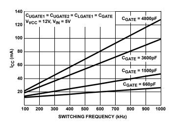
FIGURE 5. BIAS SUPPLY CURRENT vs FREQUENCY
