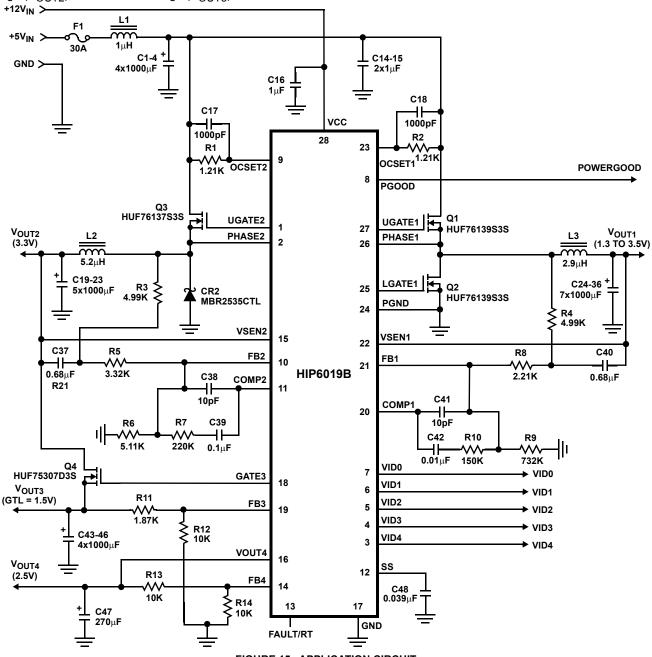
FIGURE 15. APPLICATION CIRCUIT
