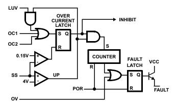
FIGURE 7. FAULT LOGIC - SIMPLIFIED SCHEMATIC
