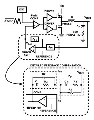
FIGURE 11. VOLTAGE-MODE BUCK CONVERTER **COMPENSATION DESIGN**
