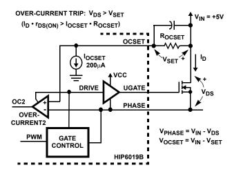
FIGURE 9. OVER-CURRENT DETECTION
