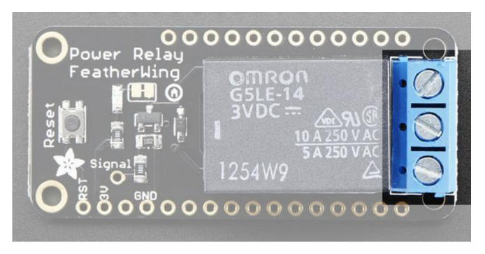
The Wing has the power control output on the end, a 3-pin 5.08 mm terminal block. The
