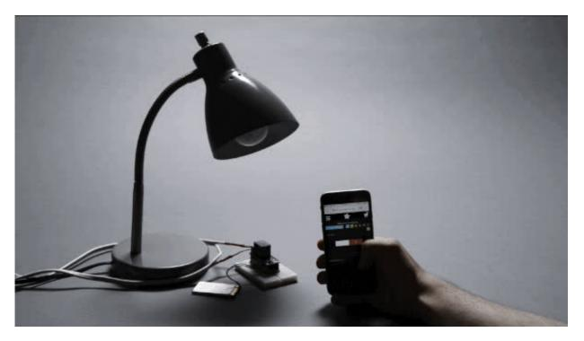
A Feather board without ambition is a Feather board without FeatherWings! This is the **Power Relay FeatherWing**. It gives you power to control, and control over power. Put simply, you can now turn on and off lamps, fans, solenoids, and other small appliances that run on up to 250VAC or DC power using any Feather board. Compared to our smaller mini Relay FeatherWings (http://adafru.it/pXA), this one can handle a beefy 1200 Watts!
