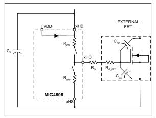
FIGURE 7-1: MIC4606 Driving an External MOSFET.
