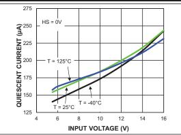
FIGURE 3-1: V<sub>DD</sub> Quiescent Current vs. Input Voltage.
