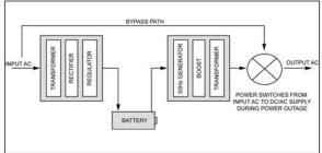
FIGURE 7-11: Type I Inverter Topology.
