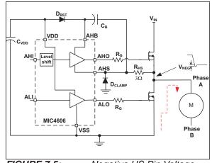
FIGURE 7-5: Negative HS Pin Voltage.
