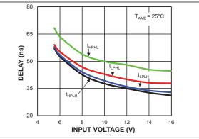
FIGURE 3-5: Propagation Delay vs. Input Voltage.
