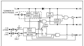
FIGURE 5-1: MIC4606 xPhase Top Level Block Diagram.
