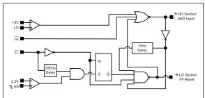
FIGURE 7-3: Adaptive Dead Time Logic Diagram.
