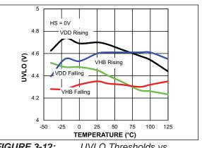
**FIGURE 3-12:** UVLO Thresholds vs. Temperature.
