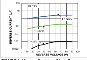
FIGURE 3-19: Bootstrap Diode Reverse Current.
