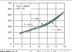
FIGURE 3-3: Input Voltage.
