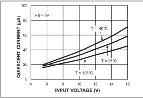
FIGURE 3-2: Shutdown Current vs. Input Voltage.
