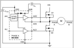
FIGURE 6-3: MIC4606 Motor Driver Example.
