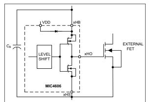
FIGURE 6-2: High-Side Driver and Bootstrap Circuit Block Diagram.
