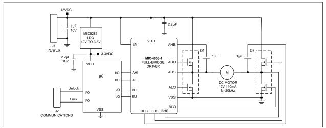
FIGURE 7-2: Door Lock/Unlock Circuit.
