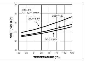
FIGURE 3-11: Low Level Output Resistance vs. Temperature.
