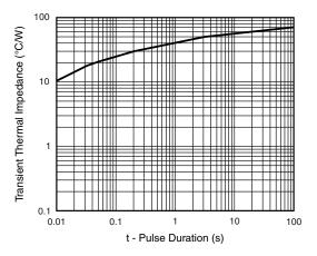
Fig. 6 - Typical Transient Thermal Impedance
