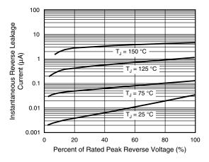
Fig. 4 - Typical Reverse Characteristics
