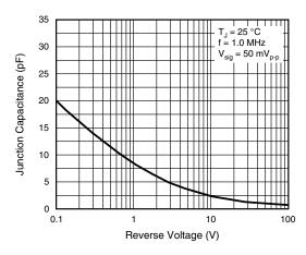
Fig. 5 - Typical Junction Capacitance
