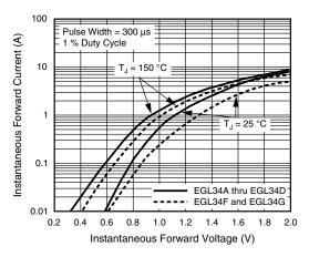
Fig. 3 - Typical Instantaneous Forward Characteristics
