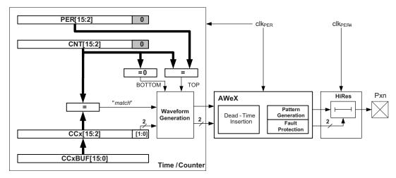
When the hi-res extension is enabled, the timer/counter must run from a non-prescaled peripheral clock. The timer/counter will ignore its two least-significant bits (lsb) in the counter, and counts by four for each peripheral clock cycle. Overflow/underflow and compare match of the 14 most-significant bits (msb) is done in the timer/counter. Count and compare of the two lsb is handled and compared in the hi-res extension running from the peripheral 4x clock.
