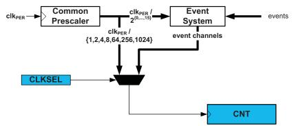
The peripheral clock ( $clk_{PER}$ ) is fed into the common prescaler (common for all timer/counters in a device). A selection of prescaler outputs from 1 to 1/1024 is directly available. In addition, the whole range of time prescalings from 1 to 2<sup>15</sup> is available through the event system.
