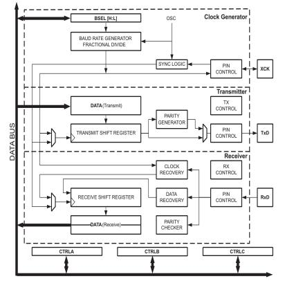
The clock generator includes a fractional baud rate generator that is able to generate a wide range of USART baud rates from any system clock frequencies. This removes the need to use an external crystal oscillator with a specific frequency to achieve a required baud rate. It also supports external clock input in synchronous slave operation.
