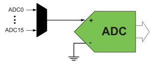
In unsigned mode, the negative input is connected to half of the voltage reference (VREF) voltage minus a fixed offset. The nominal value for the offset is:
