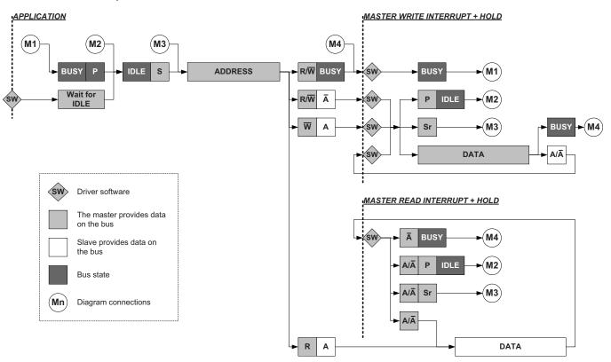
The number of interrupts generated is kept to a minimum by automatic handling of most conditions. Quick command and smart mode can be enabled to auto-trigger operations and reduce software complexity.
