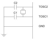
Two capacitors, C1 and C2, may be added to match the required load capacitance for the connected crystal. For details on recommended TOSC characteristics and capacitor load, refer to device datasheets.
