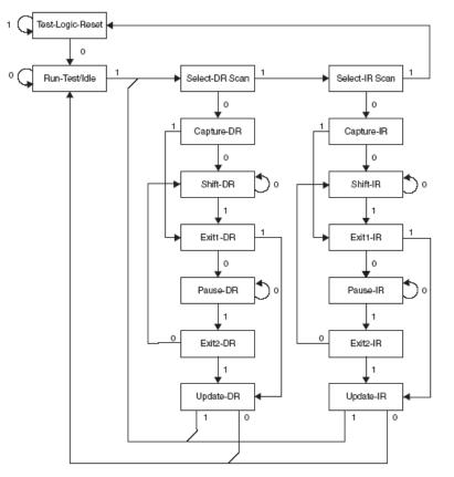
The TAP controller is a 16-state, finite state machine that controls the operation of the boundary scan circuitry. The state transitions shown in Figure 28-1 depend on the signal present on TMS (shown adjacent to each state transition) at the time of the rising edge on TCK. The initial state after a power-on reset is the test logic reset state.
