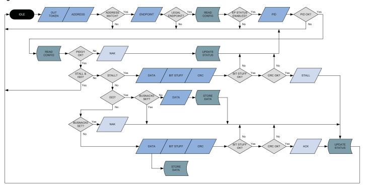
The USB module then fetches the endpoint DATAPTR register and waits for a DATA0 or DATA1 packet. If a PID error or any other PID than DATA0 or DATA1 is detected, the USB module returns to idle and waits for the next token packet.
