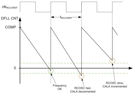
The DFLL will stop when entering a sleep mode where the oscillators are stopped. After wake up, the DFLL will continue with the calibration value found before entering sleep. The reset value of the DFLL calibration register can be read from the production signature row.
