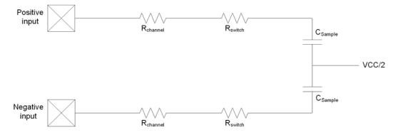
In order to achieve *n* bits of accuracy, the source output resistance, R<sub>source</sub>, must be less than the ADC input resistance on a pin:
