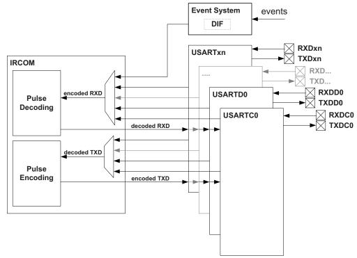
The IRCOM is automatically enabled when a USART is set in IRCOM mode. The signals between the USART and the RX/TX pins are then routed through the module as shown in Figure 22-1 on page 282. The data on the TX/RX pins are the inverted value of the transmitted/received infrared pulse. It is also possible to select an event channel from the event system as input for the IRCOM receiver. This will disable the RX input from the USART pin.
