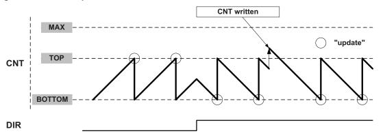
As shown in Figure 13-6, it is possible to change the counter value when the counter is running. The write access has higher priority than count, clear, or reload, and will be immediate. The direction of the counter can also be changed during normal operation.
