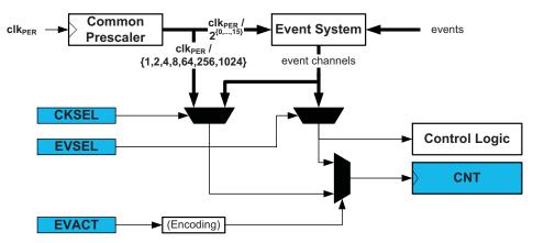
The peripheral clock is fed into a common prescaler (common for all timer/counters in a device). Prescaler outputs from 1 to 1/1024 are directly available for selection by the timer/counter. In addition, the whole range of prescaling from 1 to 2<sup>15</sup> times is available through the event system.
