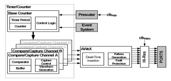
Figure 13-1. 16-bit timer/counter and closely related peripherals.
