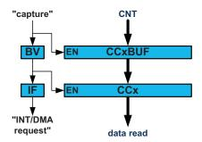
Both the CCx and CCxBUF registers are available as an I/O register. This allows initialization and bypassing of the buffer register and the double buffering function.
