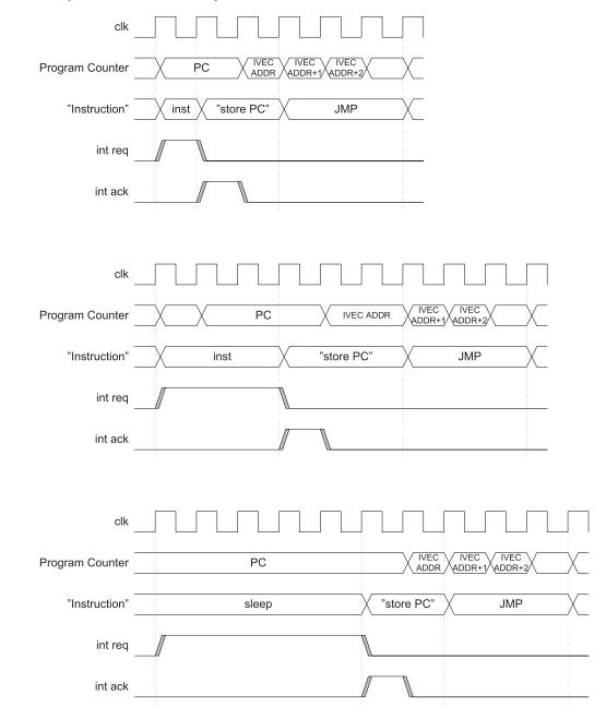
Figure 11-2. Interrupt execution of a multicycle instruction.
