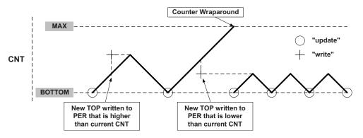
When double buffering is used, the buffer can be written at any time and still maintain correct operation. The period register is always updated on the UPDATE condition, as shown for dual-slope operation in Figure 13-9. This prevents wraparound and the generation of odd waveforms.
