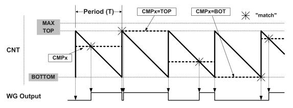
The PER register defines the PWM resolution. The minimum resolution is two bits (PER=0x0003), and the maximum resolution is eight bits (PER=MAX).
