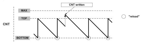
As shown in Figure 14-3, the counter can change the counter value while running. The write access has higher priority than the count clear, and reloads and will be immediate.
