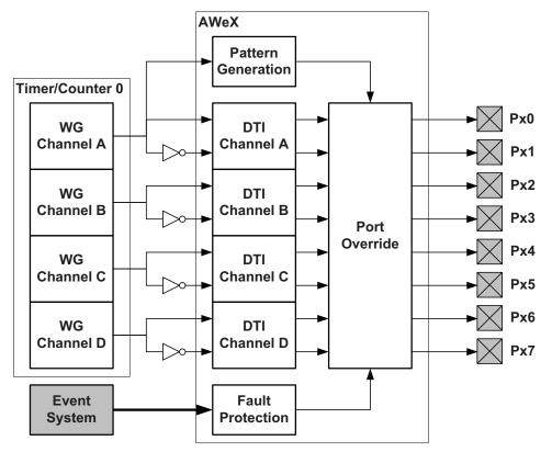
As shown in Figure 15-1 on page 185, each of the waveform generator outputs from timer/counter 0 are split into a complimentary pair of outputs when any AWeX features are enabled. These output pairs go through a dead-time insertion (DTI) unit that generates the non-inverted low side (LS) and inverted high side (HS) of the WG output with dead-time insertion between LS and HS switching. The DTI output will override the normal port value according to the port
