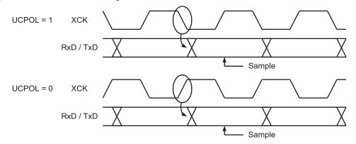
Using the inverted I/O (INVEN) setting for the corresponding XCK port pin, the XCK clock edges used for data sampling and data change can be selected. If inverted I/O is disabled (INVEN=0), data will be changed at the rising XCK clock edge and sampled at the falling XCK clock edge. If inverted I/O is enabled (INVEN=1), data will be changed at the falling XCK clock edge. For more details, see "I/O Ports" on page 123.
