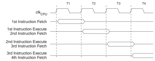
Figure 3-3 on page 9 shows the internal timing concept for the register file. In a single clock cycle, an ALU operation using two register operands is executed and the result is stored back to the destination register.
