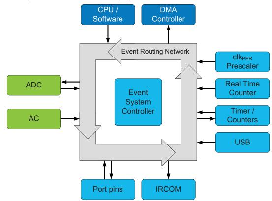
The event routing network consists of four software-configurable multiplexers that control how events are routed and used. These are called event channels, and allow for up to four parallel event configurations and routings. The maximum routing latency is two peripheral clock cycles. The event system works in both active mode and idle sleep mode.
