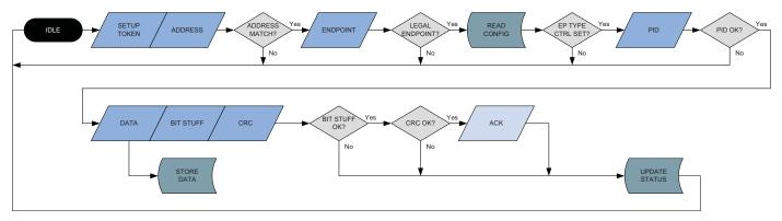
The USB module then fetches the endpoint data pointer register (DATAPTR) and waits for a DATA0 packet. If a PID error or any other PID than DATA0 is detected, the USB module returns to idle and waits for the next token packet.
