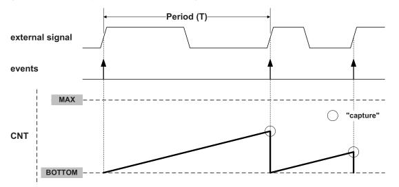
Figure 13-12. Frequency capture of an external signal.
