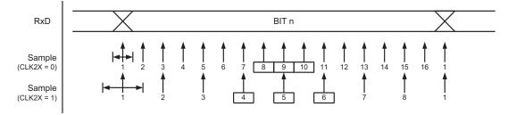
As for start bit detection, an identical majority voting technique is used on the three center samples for deciding of the logic level of the received bit. The process is repeated for each bit until a complete frame is received. It includes the first stop bit, but excludes additional ones. If the sampled stop bit is a 0 value, the frame error (FERR) flag will be set.
