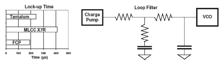
In PLL circuit applications, FCP SMT film capacitor advantages are tight tolerance on the capacitance value, stable capacitance with temperature, faster lock-up times, and no noise due to piezoelectric effects.
