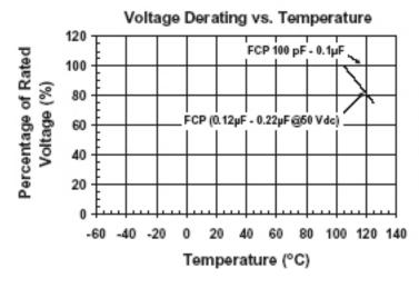
If the temperature on the surface of the capacitor is above 105°C, then the maximum voltage for FCP 50 Vdc ratings from .12 µF to .22µF must be derated linearly from full rated voltage at 105°C to 75% of the rated voltage at 125°C.
