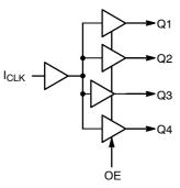
Figure 1. Block Diagram
