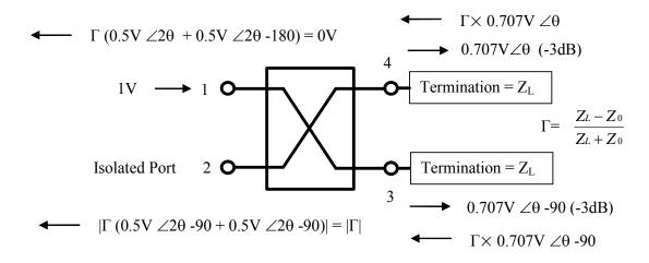
The reflection property of common mismatches in 3dB couplers is very beneficial to the operation of many networks. For instance, when splitter/combiner networks are employed to increase output power by paralleling transistors with similar reflection coefficients, input return loss is not degraded by the match of the transistor circuit. The reflections from the transistor circuits are directed away from the input to the termination at the isolated port of the coupler.
