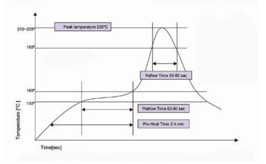
Figure 5 – Low Temperature Solder Reflow Thermal Profile
