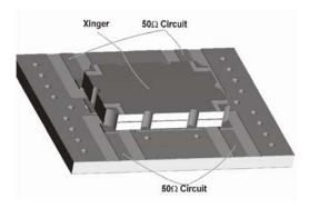
Figure 3: Component Placement
