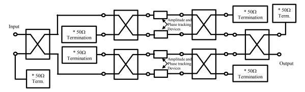
The splitter/combiner networks illustrated above use only 3dB (hybrid) couplers and are limited to binary divisions (2<sup>n</sup> number of splits, where *n* is an integer). Splitter/combiner circuits configured this way are known as "corporate" networks. When a non-binary number of divisions is required, a "serial" network must be used. Serial networks can be designed with [3, 4, 5, ...., n] splits, but have a practical limitation of about 8 splits.
