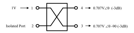
The hybrid coupler can also be used to combine two signals that are applied with equal amplitudes and phase quadrature (90° phase difference). An example of this function is illustrated below.
