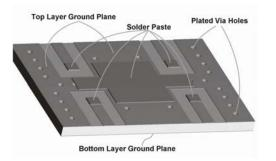
**Reflow:** The surface mount coupler is conducive to most of today's conventional reflow methods. A low and high temperature thermal reflow profile are shown in Figures 5 and 6, respectively. Manual soldering of these components can be done with conventional surface mount non-contact hot air soldering tools. Board pre-heating is highly recommended for these selective hot air soldering methods. Manual soldering with conventional irons should be avoided.
