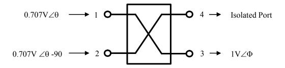
3dB couplers have applications in circuits which require splitting an applied signal into 2, 4, 8 and higher binary outputs. The couplers can also be used to combine multiple signals (inputs) at one output port. Some splitting and combining schemes are illustrated below:
