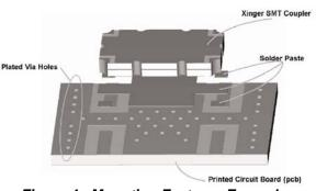
Figure 4: Mounting Features Example
