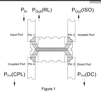
The coupler is excited at the input port with  $P_{in}$  (watts) of power. Assuming the coupler is not ideal, and that there are no radiation losses, power will exit the coupler at all four ports. Symbolically written,  $P_{out(RL)}$  is the power that is returned to the source because of impedance mismatch,  $P_{out(ISO)}$  is the power at the isolated port,  $P_{out(CPL)}$  is the power at the coupled port, and  $P_{out(DC)}$  is the power at the direct port.
