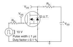
Fig. 10a - Switching Time Test Circuit
