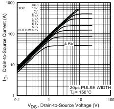
Fig. 2 - Typical Output Characteristics
