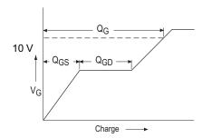
Fig. 13a - Basic Gate Charge Waveform
