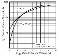
Fig. 3 - Typical Transfer Characteristics
