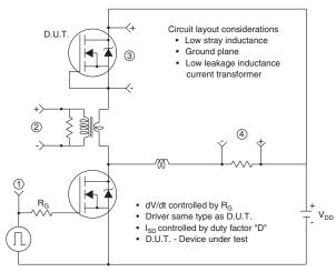
Fig. 13c - Peak Diode Recovery dV/dt Test Circuit
