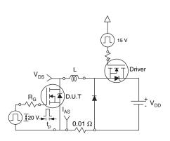
Fig. 12a - Unclamped Inductive Test Circuit
