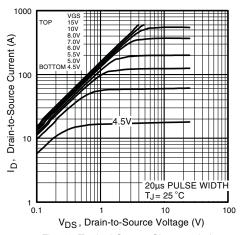
Fig. 1 - Typical Output Characteristics
