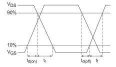
Fig. 10b - Switching Time Waveforms
