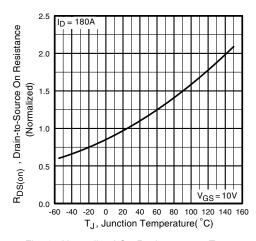
Fig. 4 - Normalized On-Resistance vs. Temperature
