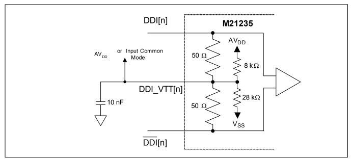
Figure 2-2. Input circuit for M21235
