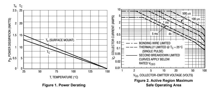
There are two limitations on the power handling ability of a transistor: average junction temperature and second breakdown. Safe operating area curves indicate  $I_C-V_{CE}$  limits of the transistor that must be observed for reliable operation; i.e., the transistor must not be subjected to greater dissipation than the curves indicate.
