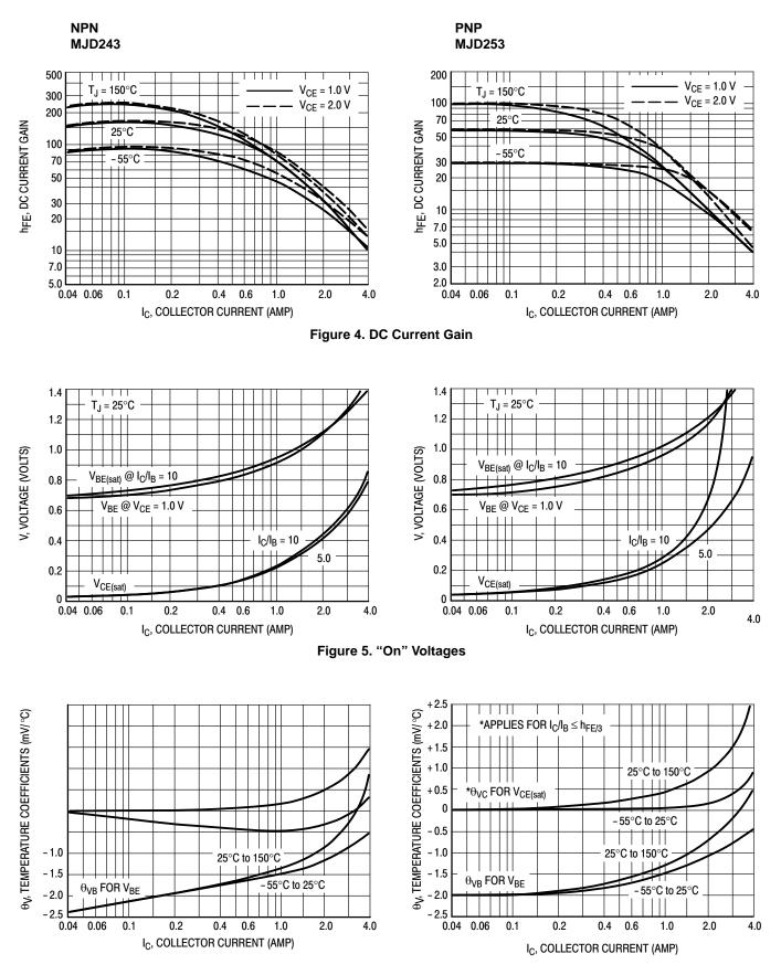
Figure 6. Temperature Coefficients
