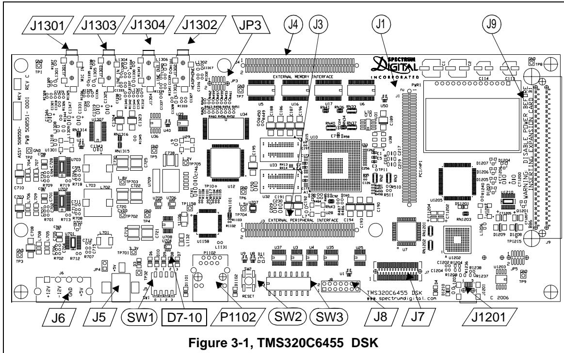
Figure 3-1, TMS320C6455 DSK
