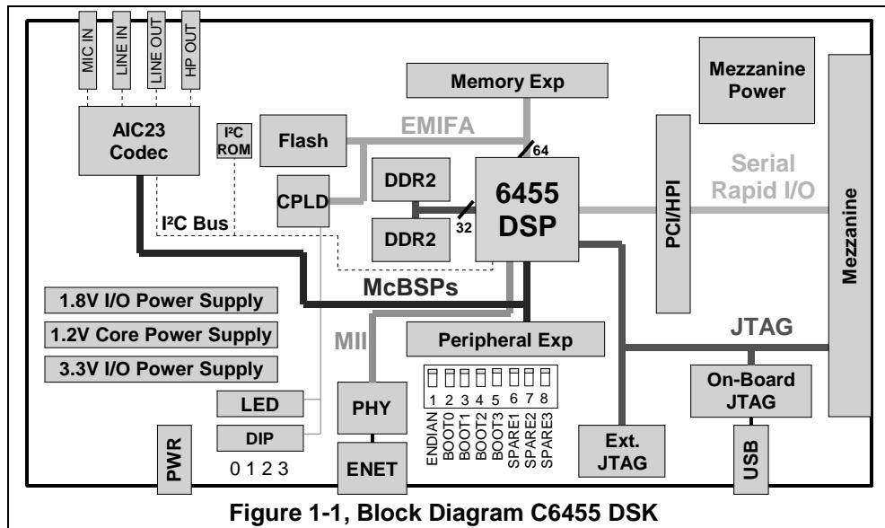
The DSK comes with a full compliment of on-board devices that suit a wide variety of application environments. Key features include:
