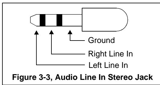
**Figure 3-3, Audio Line In Stereo Jack**
