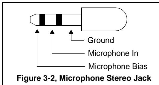
**Figure 3-2, Microphone Stereo Jack**
