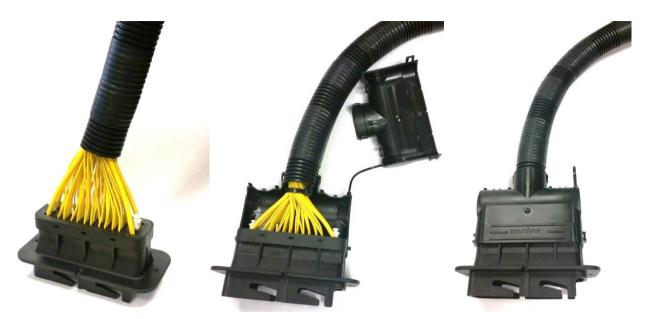
Figure 4.34: (Left) A fully-assembled SRC Male Connector Assembly with conduit around the wires, (Middle) one half of the Conduit Interface assembled with a tie wrap used as strain relief on the cables and (Right) a correctly assembled conduit to a SRC Male Connector using the appropriate Conduit Interface
