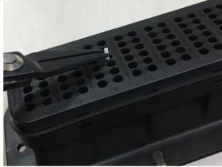
Figure 4.43a shows a method of gripping blind cavity plug in male connector prior to it being snipped (if placed in incorrect circuit position)
