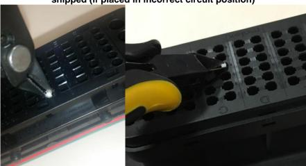
Figure 4.43b shows a method of gripping blind cavity plug after it has been snipped
