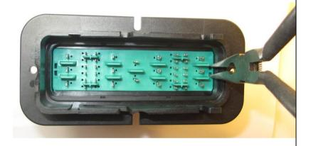
Figure 4.39: Moving the TPA on the Male Connector Assembly to the Pre-Load Position
