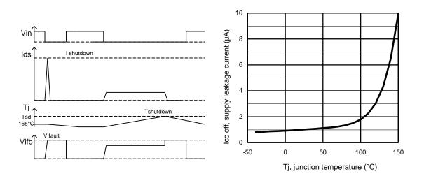
Figure 3 – Protection timing diagram
