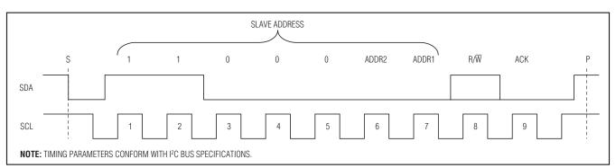
Figure 1. MAX3540 Slave Address Byte
