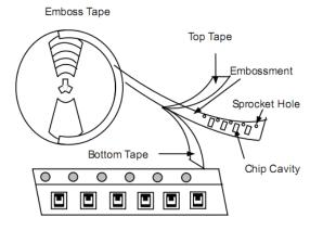
Note: The sprocket holes are to the right as the tape is pulled toward the user.
