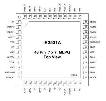
Figure 2: IR3531A Package Top View
