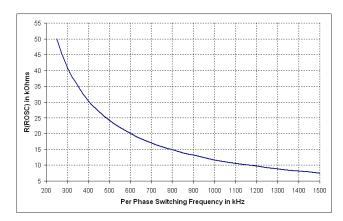
Figure 17: RROSC vs. Per-phase Switching Frequency
