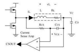
Figure 9: Inductor Current Sensing and Current Sense Amplifier
