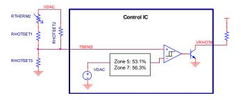
**Figure 15: Over Temperature Detection Circuit**
