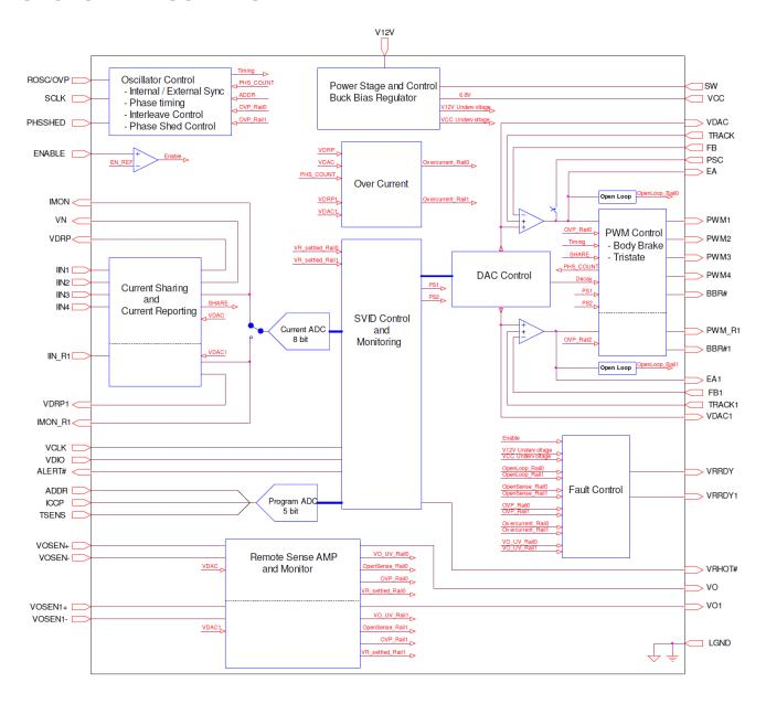
Figure 4: IR3531A Block Diagram
