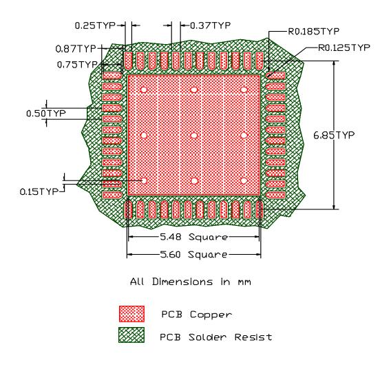
Figure 20: Solder Resist
