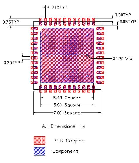
**Figure 19: Metal and Component Placement**
