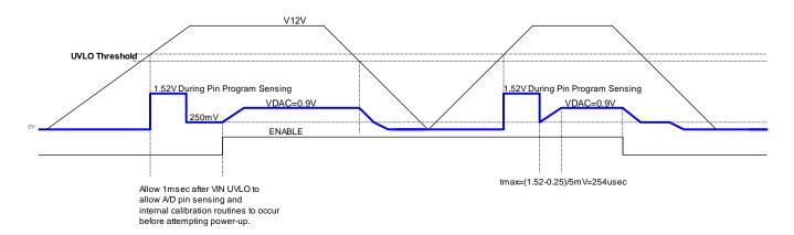
Figure 12: V12V Power and Enable Cycling
