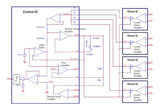
Figure 10: Adaptive voltage positioning with thermal compensation
