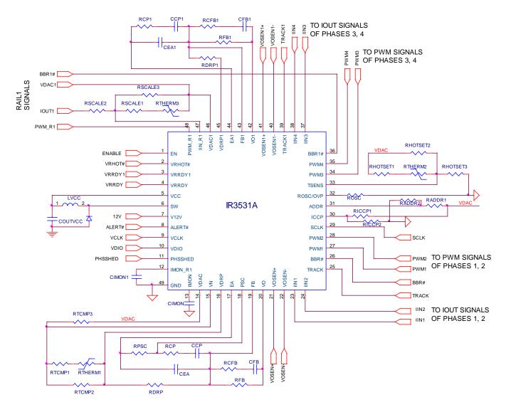
Figure 5: IR3531A Typical Application Diagram
