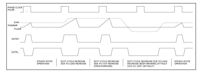
**Figure 8: PWM Operating Waveforms**
