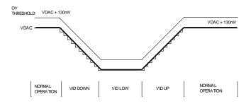
Figure 16: Over Voltage Protection during SETVID Fast/Slow
