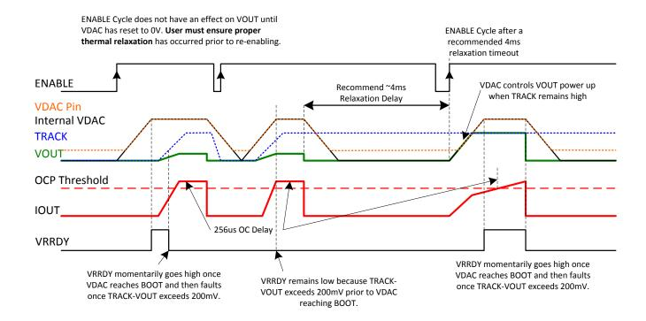
**Figure 14: Over Current Waveforms**
