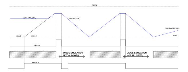
Figure 13: Enable Power Cycling Under Pre-bias
