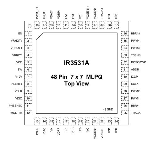
Figure 3: Package Top View, Enlarged
