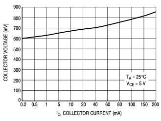
Figure 3. Collector Saturation Region
