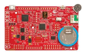
This kit features a PSoC 4000S device with a CapSense trackpad, buttons, and a proximity loop. The board includes an on-board 1Mbit F-RAM, an EZ-BLE™ PRoCTM module, and a rechargeable coin-cell battery.
