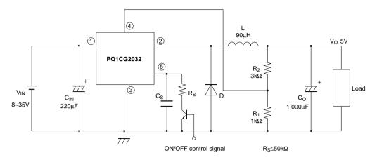
Fig.16 Polarity Inversion Type Circuit Diagram
