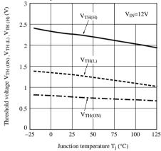
Fig.11 Overcurrent Detecting Level Fluctuation vs. Junction Temperature
