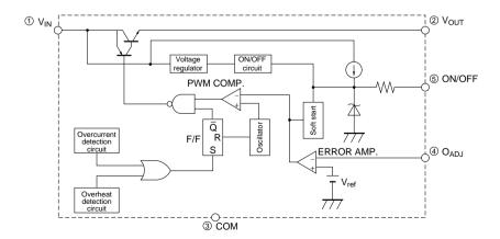
Fig.15 Step Down Type Circuit Diagram
