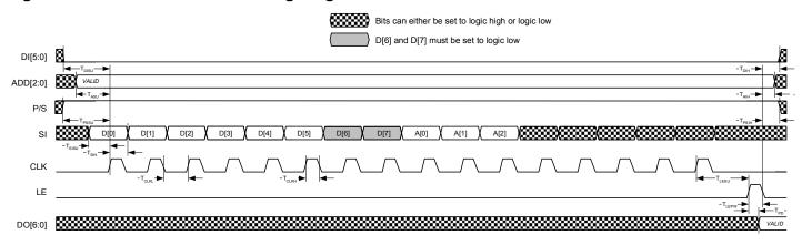
Figure 21. Latched-Parallel/Direct-Parallel Timing Diagram
