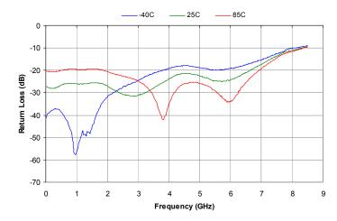
Figure 11. Output Return Loss vs. Temperature: 15.75 dB State
