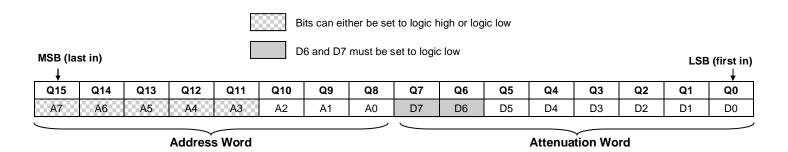
Attenuation Word is derived directly from the attenuation value. For example, to program the 12.75 dB state at address 3:
