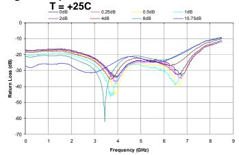
Figure 9. Output Return Loss vs. Attenuation: T = +25C
