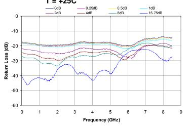
Figure 10. Input Return Loss vs. Temperature: 15.75 dB State
