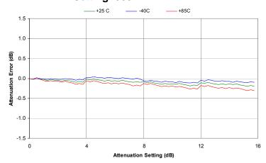
Figure 15. Attenuation Error vs. Attenuation Setting: 1800 MHz
