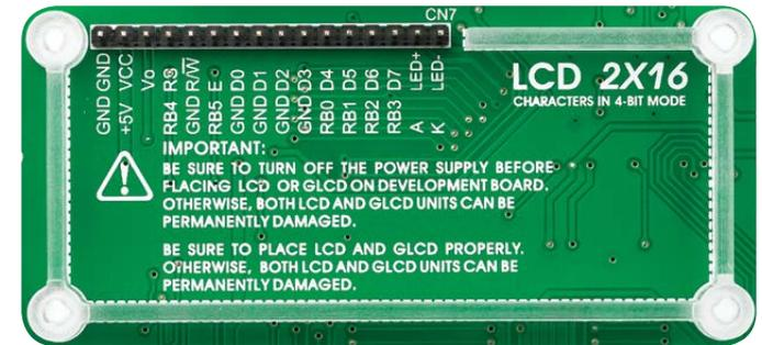
Figure 11-1: On-board LCD 2x16 display connector
