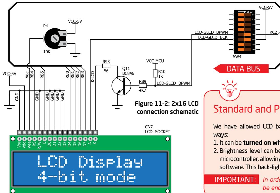
Figure 11-2: 2x16 LCD connection schematic
