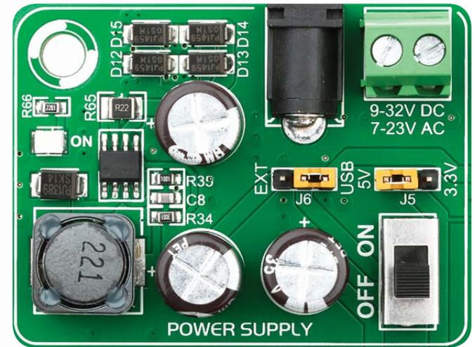
Figure 3-1: Dual power supply unit of EasyPIC™ v7
