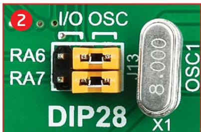
**Figure 4-7:** RA6 and RA7 connected to X1 quartz-crystal
