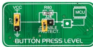
**Figure 10-5:** Button press level jumper (J17)
