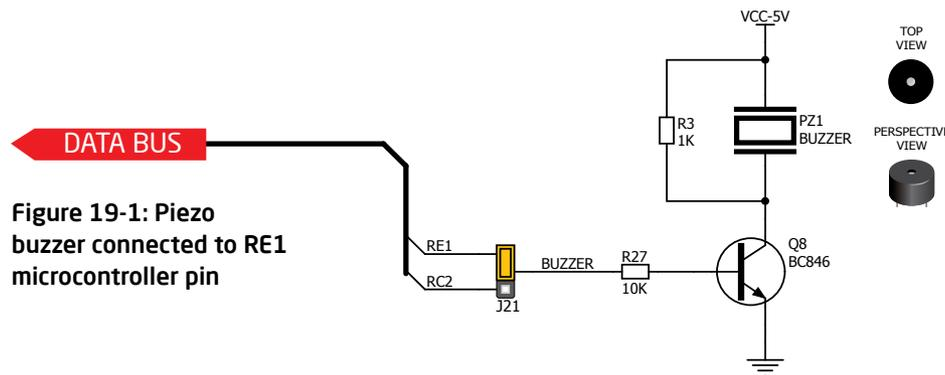
Figure 19-1: Piezo buzzer connected to RE1 microcontroller pin
