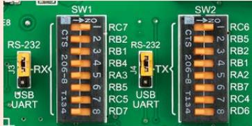
In order to enable RS-232 communication, you must set **J3** and **J4** jumpers in the **RS-232** position, and enable desired **RX** and **TX** lines via **SW1** and **SW2** DIP switches. For example, if you want to enable RS-232 connection on UART1 module of the default **PIC18F45K22** chip, you should enable **SW1.1** (RC7) and **SW2.1** (RC6) lines.
