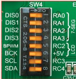
**Figure 18-1:** Activate SW4.7 and SW4.8 switches to connect microcontroller I<sup>2</sup>C lines to Serial EEPROM.
