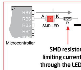
**LED (Light-Emitting Diode)** is a highly efficient electronic light source. When connecting LEDs, it is necessary to place a current limiting resistor in series so that LEDs are provided with the
