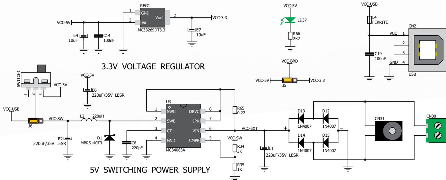
Figure 3-2: Dual power supply unit schematic
