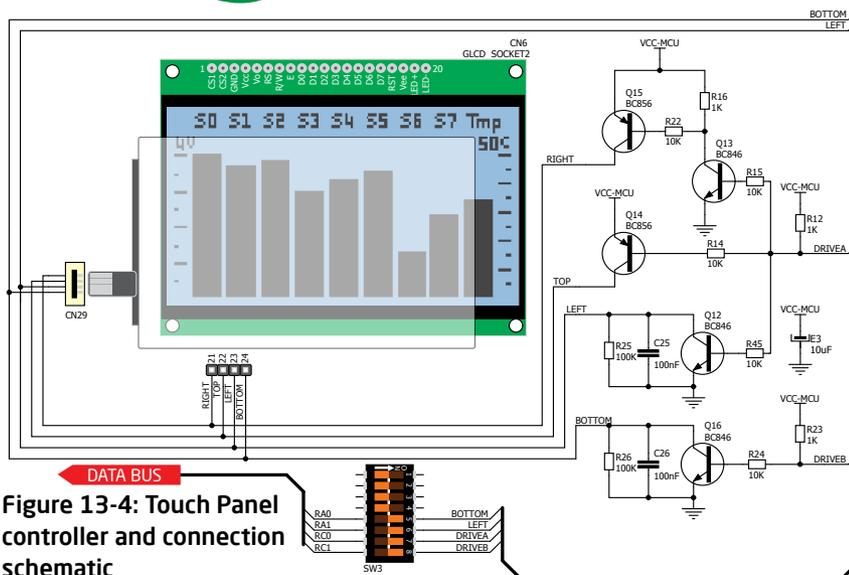
Figure 13-4: Touch Panel controller and connection schematic
