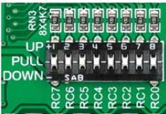
1. **middle position** disables both pull-up and pull-down feature from the PORT pin
