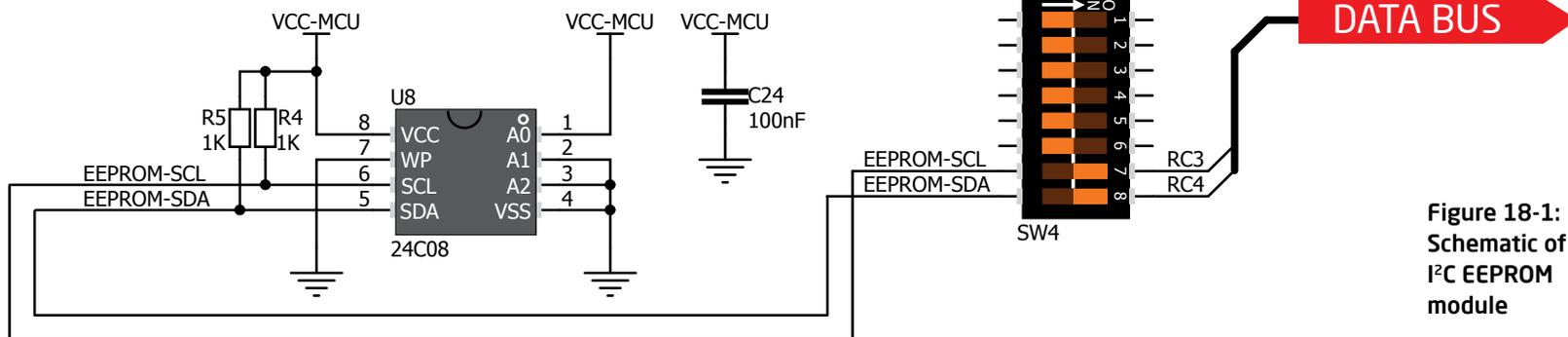
**Figure 18-1:** Schematic of I<sup>2</sup>C EEPROM module
