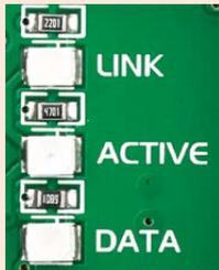
Three LEDs indicate specific programmer operation. **Link** LED lights up when USB link is established with your PC, **Active** LED lights up when programmer is active. **Data** is on when data is being transferred between the programmer and PC software (compiler or mikroProg Suite™ for PIC®).
