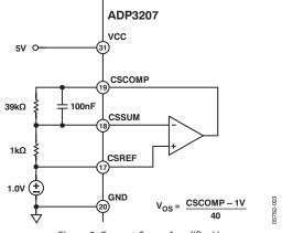
Figure 3. Current-Sense Amplifier  $V_{\text{OS}}$
