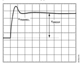
Figure 16. Transient Setting Waveform, Load Release
