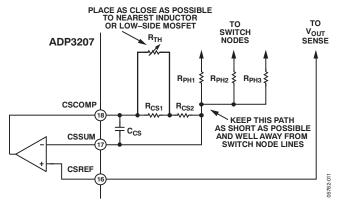
Figure 11. Temperature Compensation Circuit Values
