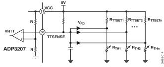
Figure 13. Multiple-Point Thermal Monitoring
