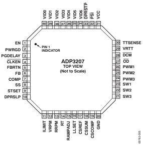
Figure 5. Pin Configuration
