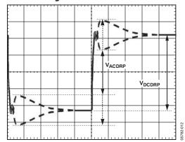
Figure 14. AC Loadline Waveform
