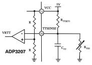
Figure 12. Single-Point Thermal Monitoring
