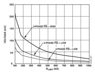
Figure 8. Current-Limit Threshold Voltage vs. RLIMIT
