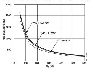
Figure 6. Master Clock Frequency vs.  $R_T$
