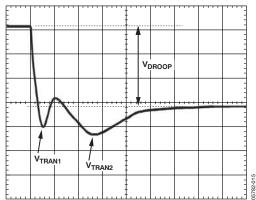
Figure 15. Transient Setting Waveform, Load Step
