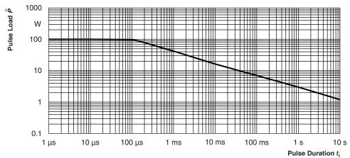
Maximum pulse load, single pulse; applicable if  $P \rightarrow 0$  and  $n \le 1000$  and  $\hat{U} \le \hat{U}_{\text{max}}$ ; for permissible resistance change  $\pm$  (0.5 % R + 0.01  $\Omega$ )
