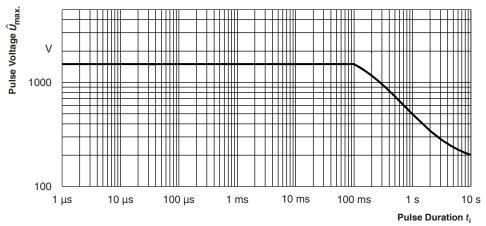
Maximum pulse voltage, single and continuous pulses; applicable if  $\hat{P} \leq \hat{P}_{\text{max}}$ ; for permissible resistance change  $\pm$  (0.5 % R + 0.01  $\Omega$ )
