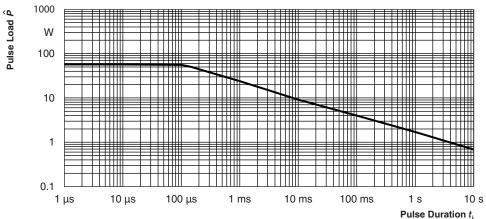
Maximum pulse load, continuous pulse; applicable if  $\vec{P} \leq P$  ( $\vartheta_{amb}$ ) and  $\hat{U} \leq \hat{U}_{max}$ ; for permissible resistance change ± (0.5 % R + 0.01  $\Omega$ )
