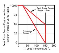
FIGURE 3 - Derating Curve
