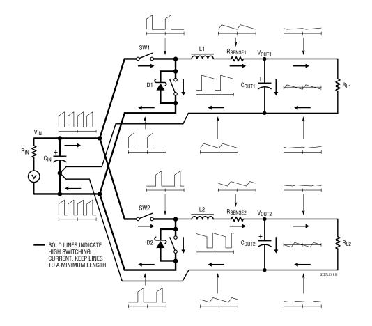
Figure 11. Branch Current Waveforms
