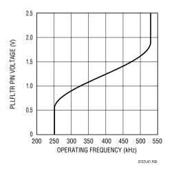
Figure 5. PLLFLTR Pin Voltage vs Frequency
