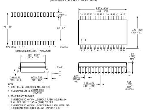
**G** Package 28-Lead Plastic SSOP (5.3mm) (Reference LTC DWG # 05-08-1640)
