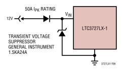
Figure 9. Automotive Application Protection
