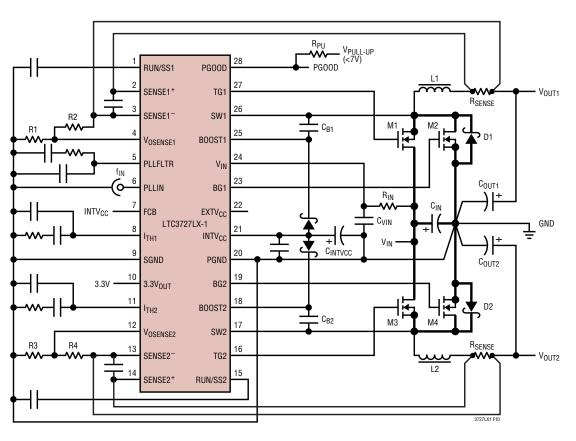
Figure 10. LTC3727LX-1 Recommended Printed Circuit Layout Diagram
