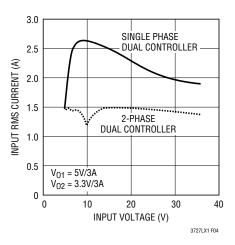
Figure 4. RMS Input Current Comparison
