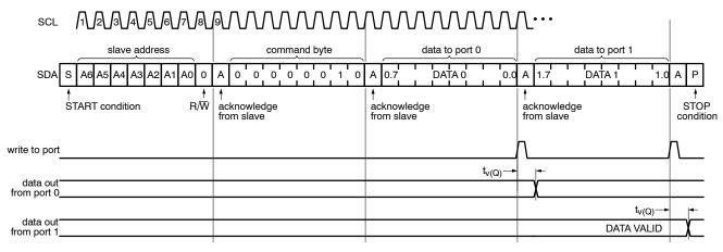
Figure 6. Write to Output Port Registers
