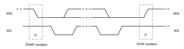
Figure 15. Definition of START and STOP Conditions
