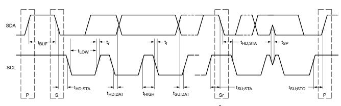
Figure 18. Definition of Timing on the I<sup>2</sup>C Bus
