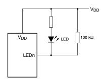
Figure 12. High Value Resistor in Parallel with the LED
