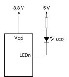
Figure 13. Device Supplied by a Lower Voltage
