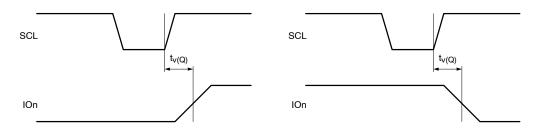
Figure 20. t<sub>V(Q)</sub> Timing
