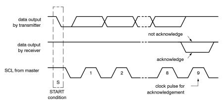
Figure 17. Acknowledgement of the I<sup>2</sup>C Bus
