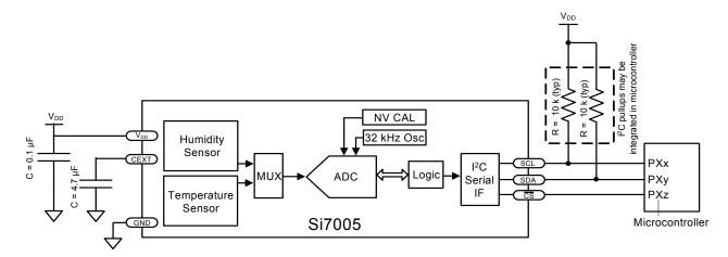
Figure 6. Si7005 Functional Block Diagram
