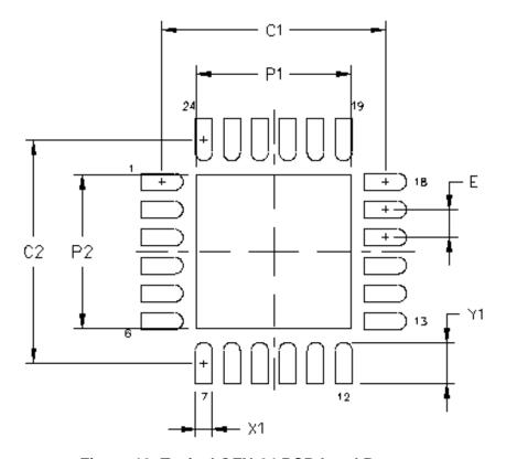
Figure 13. Typical QFN-24 PCB Land Pattern
