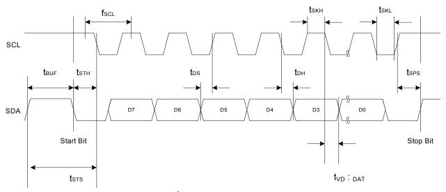
Figure 1. I<sup>2</sup>C Interface Timing Diagram
