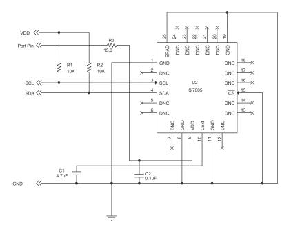
Figure 5. Typical Application Circuit for Battery-Powered Applications
