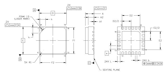
Figure 12. 24-Pin Quad Flat No Lead (QFN) With Protective Cover
