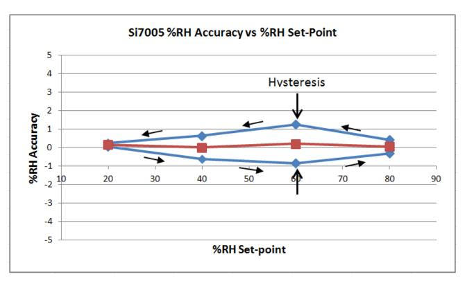
Figure 7. Measuring Sensor Accuracy Including Hysteresis
