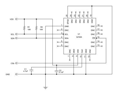
**Figure 4. Typical Application Circuit**
