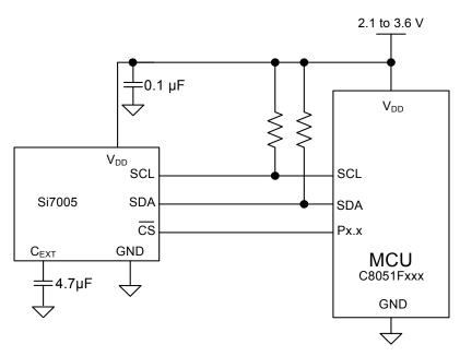
**Figure 9. Typical Connection Diagram**
