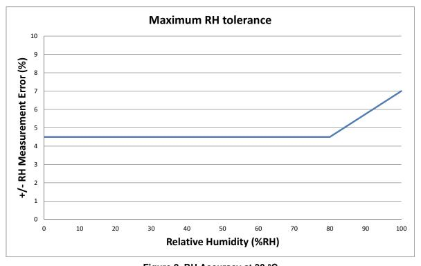
Figure 2. RH Accuracy at 30 °C
