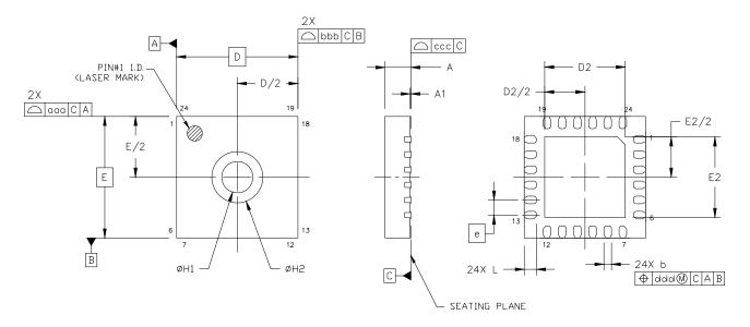
Figure 11. 24-Pin Quad Flat No Lead (QFN)
