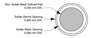
Figure 1. Recommended Non-Solder Mask Defined Pad Illustration
