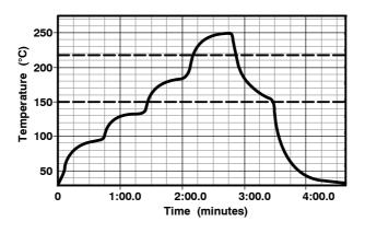
Figure 2. Lead-free (SnAgCu) Solder Ball Reflow Profile
