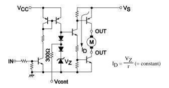
As shown in the above diagram, the Vcont pin outputs the voltage of the band gap Zener  $V_Z + V_F$  (=1.93V). In normal use, this pin is left open.
