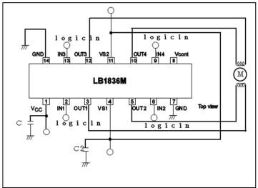
3. Example of applied circuit when connecting it in parallel The use likened to H bridge 1ch is shown possible in the figure below by connecting IN1 with IN3, IN2 with IN4, OUT1 with OUT3, OUT2, and OUT4. (IO max=2.0A, Upper and lower total  $R_{ON}$ =0.5 $\Omega$ )
