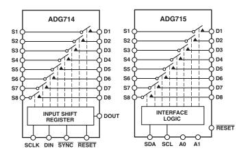
On power-up of these devices, all switches are in the OFF condition, and the internal registers contain all zeros.
