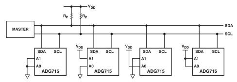
Figure 6. Multiple ADG715s On One Bus
