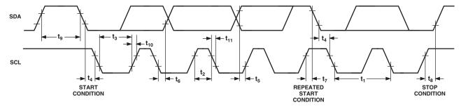
Figure 2. 2-Wire Serial Interface Timing Diagram
