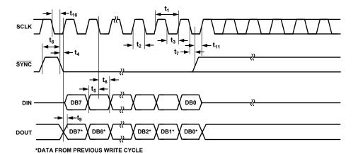
Figure 1. 3-Wire Serial Interface Timing Diagram
