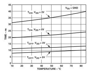
TPC 15. T<sub>ON</sub>/T<sub>OFF</sub> Times vs. Temperature for ADG714
