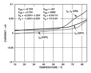
TPC 9. Leakage Currents as Function of Temperature
