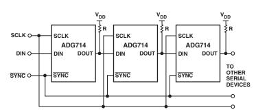
Figure 7. Multiple ADG714 Devices in a Daisy-Chained Configuration
