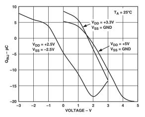
TPC 14. Charge Injection vs. Source/Drain Voltage
