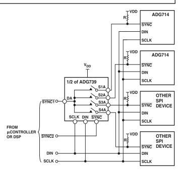
Figure 8. Addressing Multiple ADG714s Using an ADG739
