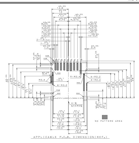
NOTE1.Card Frictional locking function is available for inserted SD card only but not for MMC.
