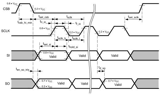
Figure 4. SPI Signals Timing Parameters
