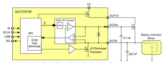
Figure 7. Electro Chromic Mirror Application Diagram
