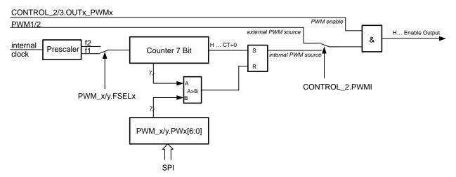
Figure 5. PWM Generation Diagram
