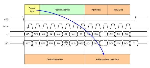
Figure 10. SPI Frame Format
