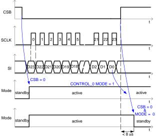
Figure 9. Mode Timing Diagram
