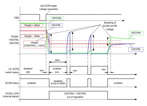
Figure 6. PWM Discharge Mode for ECFB
