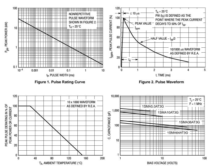
Figure 3. Pulse Derating Curve
