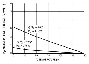
Figure 5. Steady State Power Derating
