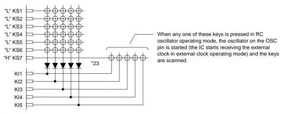
Note: \*23. These diodes are required to reliably recognize multiple key presses on the KS7 line when sleep mode state with only KS7 high, as in the above example.
