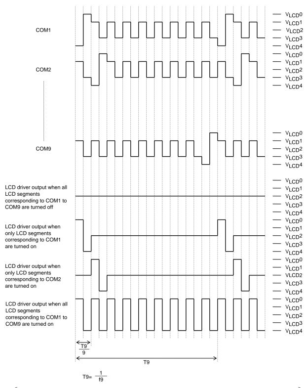
When a "set display technique" instruction with FC0 = 0, FC1 = 0 are executed:  $f9 = \frac{fosc}{3456}$ ,  $f9 = \frac{fCK}{3456}$ When a "set display technique" instruction with FC0 = 1, FC1 = 0 are executed:  $f9 = \frac{fosc}{1728}$ ,  $f9 = \frac{fCK}{1728}$ When a "set display technique" instruction with FC0 = 0, FC1 = 1 are executed:  $f9 = \frac{fosc}{864}$ ,  $f9 = \frac{fCK}{864}$
