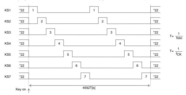
Note: \*22. Not that the high/low states of these pins are determined by the "set key scan output port/general-purpose output port state" instruction, and that key scan output signals are not output from pins that are set to low.
