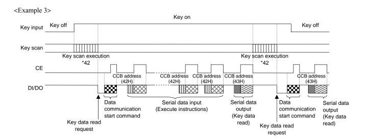
Note: \*42. When the key data agrees for two key scans, the key scan execution time is 4800T[s].
