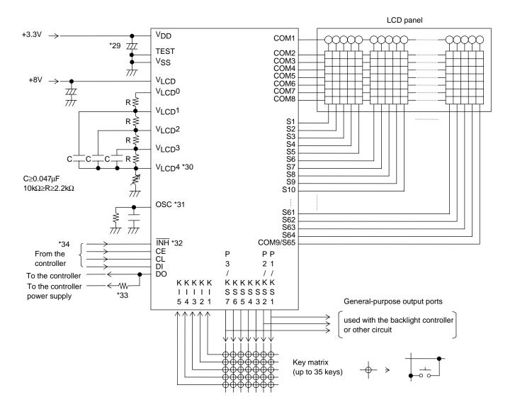
Note \*29. Add a capacitor to the logic block power supply line so that the logic block power supply voltage V<sub>DD</sub> rise time when power is applied and the logic block power supply voltage V<sub>DD</sub> fall time when power drops are both at least 1 ms, as the LC75812PT is reset by the V<sub>DET</sub>.
