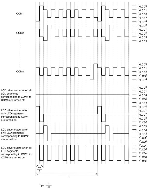
When a "set display technique" instruction with FC0 = 0, FC1 = 0 are executed:  $f8 = \frac{fosc}{3072}$ ,  $f8 = \frac{fCK}{3072}$ When a "set display technique" instruction with FC0 = 1, FC1 = 0 are executed:  $f8 = \frac{fosc}{1536}$ ,  $f8 = \frac{fCK}{1536}$ When a "set display technique" instruction with FC0 = 0, FC1 = 1 are executed:  $f8 = \frac{fosc}{768}$ ,  $f8 = \frac{fCK}{768}$
