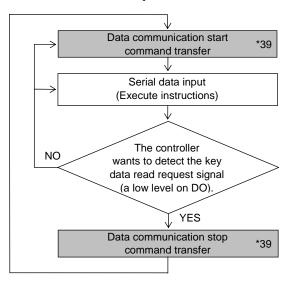
Note: \*39. In the case of the 4 line type CCB format, the transfers of data communication start command and data communication stop command are unnecessary, and, in the case of the 3 line type CCB format, these transfers are necessary.
