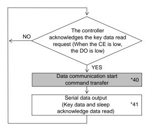
Note: \*40. In the case of the 4 line type CCB format, the transfer of data communication start command is unnecessary, and, in the case of the 3 line type CCB format, the transfer is necessary.
