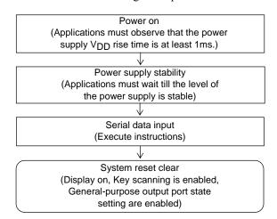
Note: The flowchart for power-on time initialization is the same for the 4- and 3-wire CCB formats. See "Power Supply Sequence" and "System Reset."
