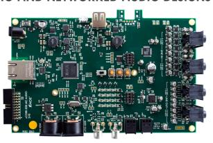
The xCORE-200 Multichannel Audio Platform and XMOS reference software provide a scalable and flexible solution for a wide range of consumer and professional audio products.
