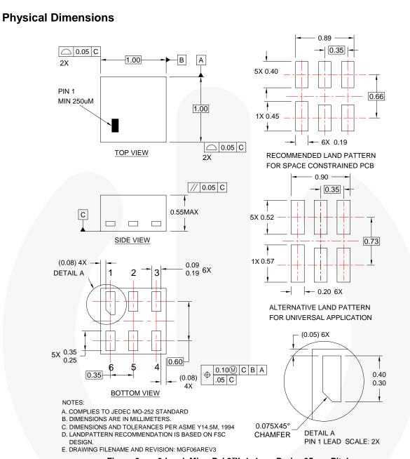
Figure 9. 6-Lead, MicroPak2™, 1x1mm Body, .35mm Pitch
