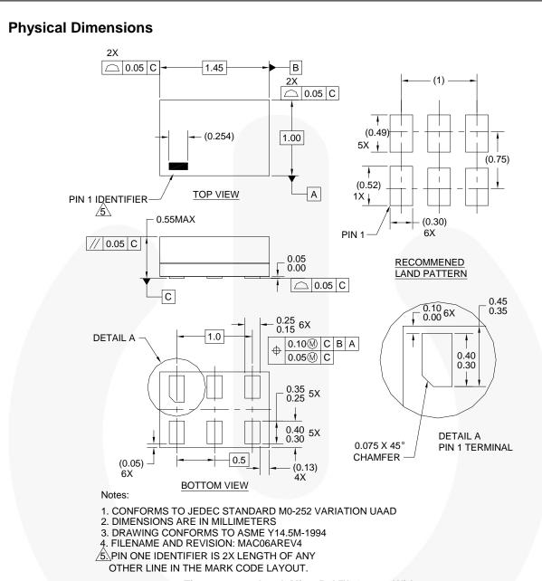
Figure 8. 6-Lead, MicroPak<sup>™</sup>, 1.0mm Wide
