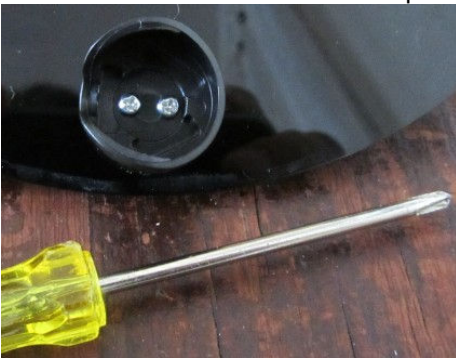
Attach the ball caster to the base plate with the two shortest screw's (on the opposite side as the motors)
