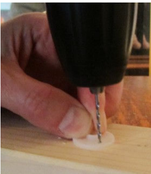
Use a 2mm drill on the 4 holes for wheel to horn assembly.
