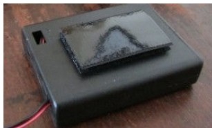
Glue Velcron to battery case
