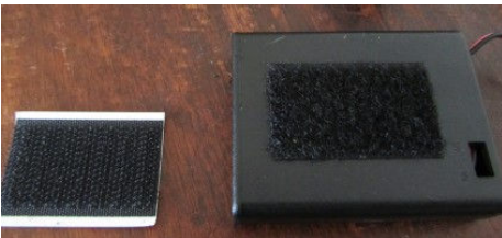
Glue Velcron to battery case
