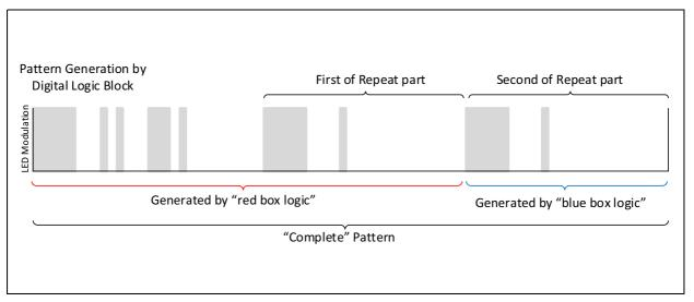
Pattern Generation: All of the "one-time" sub-pattern and the "first" instance of the "repeated" sub-pattern is actually run by the logic in the red box. The second instance of the "repeated" sub-pattern is run by the logic in the blue box.
