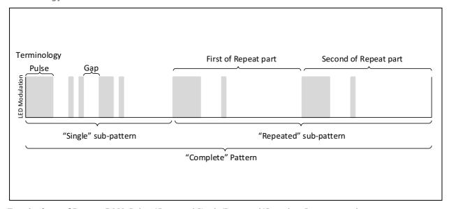
**Terminology of Pattern RAM:** Pulses/Gaps, and Single/Repeated/Complete Patterns are shown.
