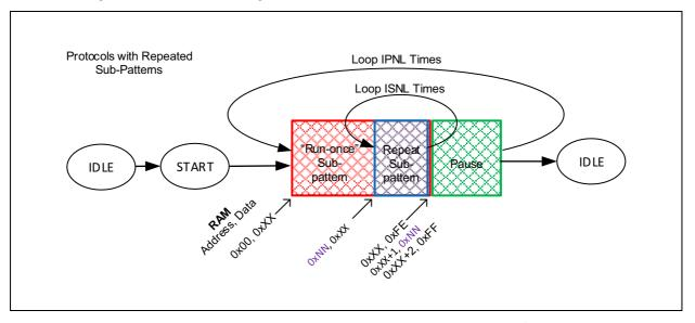
Protocols with "Repeated" Sub-Patterns: The blue box represents a repeated part of a pattern. These sub-patterns begin at an address within the red box and burst until the end of the pattern is encountered. The repeated sub-pattern can be reiterated 1 to 254 times, or continuously.
