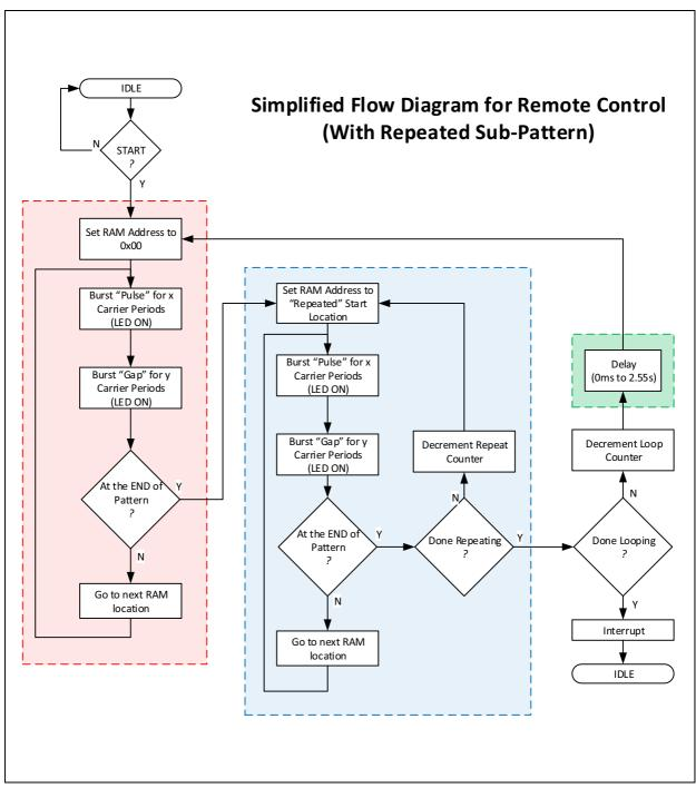
**Simplified Flow Diagram:** The digital logic in the remote control engine has been tailored to fit the data format and protocol specifications for IR remote control. "Press and Release" type buttons (E.g. Power) are generated using the logic in the red box (logic in the blue box is not needed). "Press and Hold" type buttons (E.g. Volume+) are generated using logic in both the red and blue boxes.
