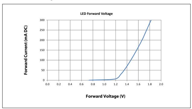
1. The voltage on the LDR pin (VLEDA – VLED FORWARD) must be sufficiently large to guarantee proper operation of the regulated current sink.
