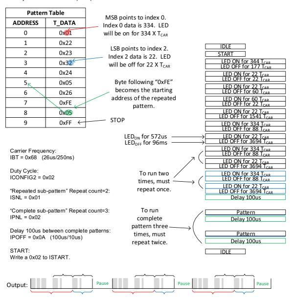
**Practical Example:** Device registers and RAM are loaded with values to generate a real remote control waveform.
