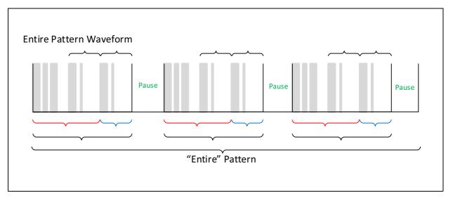
**Entire Pattern:** Complete patterns can also be separated by a pause, or time delay, as generated by the logic in the green block. The entire pattern consists of a multiple of complete patterns and pause delays. During the length of time the entire pattern is bursting, the PBUSY bit is set.
