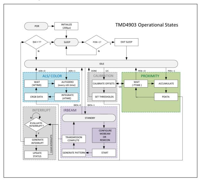
1. While IRBeam is enabled (IBEN = 1), PROXIMITY is disabled automatically.
