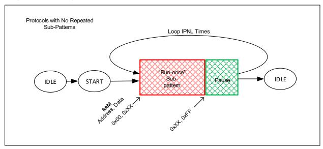
**Complete Pattern Loops:** The red box represents a "run-once" pattern. The pattern begins at pattern ram address 0x00 and bursts until the end of the pattern is encountered. The complete pattern can be reiterated 1 to 254 times, or continuously.
