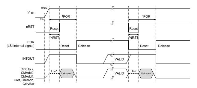
Figure 7. Power-on Sequence by the External Reset
