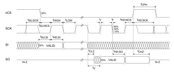
Figure 11. SPI Data Timing
