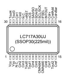
Figure 5. Pin Assignment (Top View)
