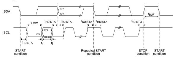
Figure 8. I<sup>2</sup>C Data Timing
