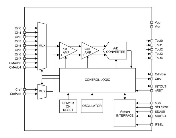
Figure 4. Simplified Block Diagram
