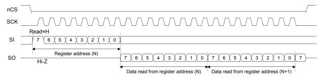
Figure 13. SPI Read Format
