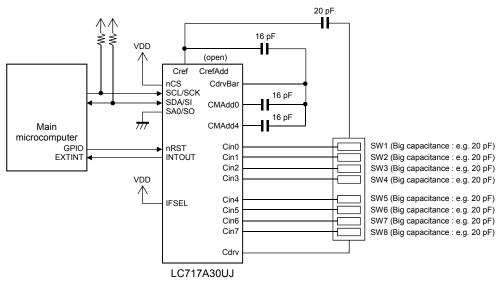
Figure 3. Application Schematic 3
