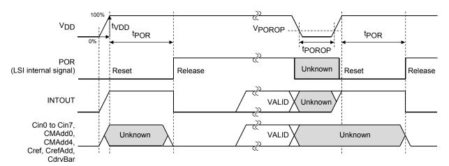
Figure 6. Power-on Sequence by the Power-on Reset
