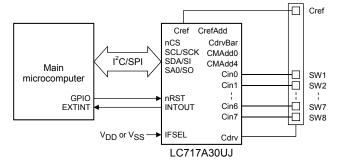
Figure 1. Application Schematic 1
