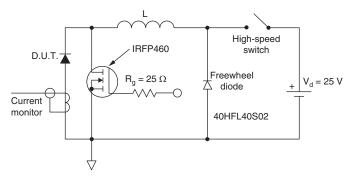
Fig. 8 - Unclamped Inductive Test Circuit
