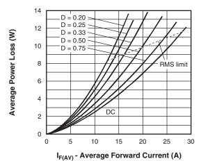
Fig. 6 - Forward Power Loss Characteristics
