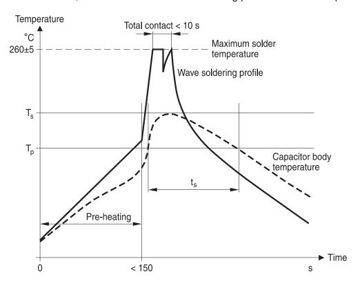
T<sub>s</sub>: Capacitor body maximum temperature at wave soldering
