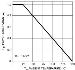
Fig. 1 Power Dissipation vs. Ambient Temperature
