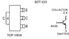
Schematic and Pin Configuration
